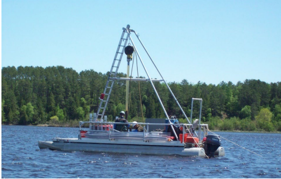
Figure 10. Photograph of the Vibracore Sampling Equipment Used to Collect 4-inch Sediment Cores for Radiometric Dating (GLEC, 2011)
